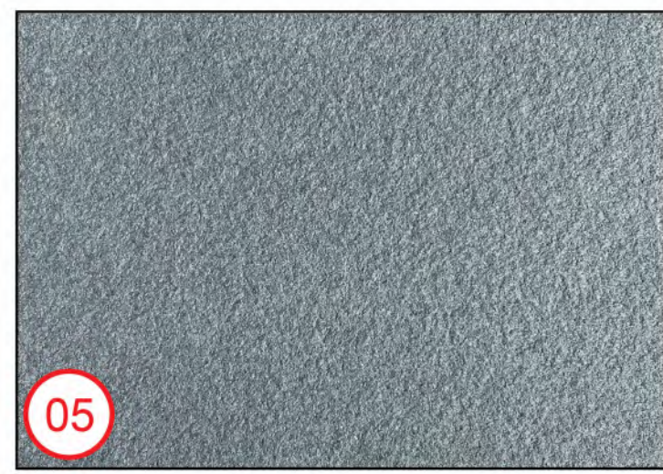
05 FIBER CEMENT PANEL RAIN SCREEN - CHARCOAL BASIS OF DESIGN: CEMBRIT PATINA ROUGH - P070 FLINT
