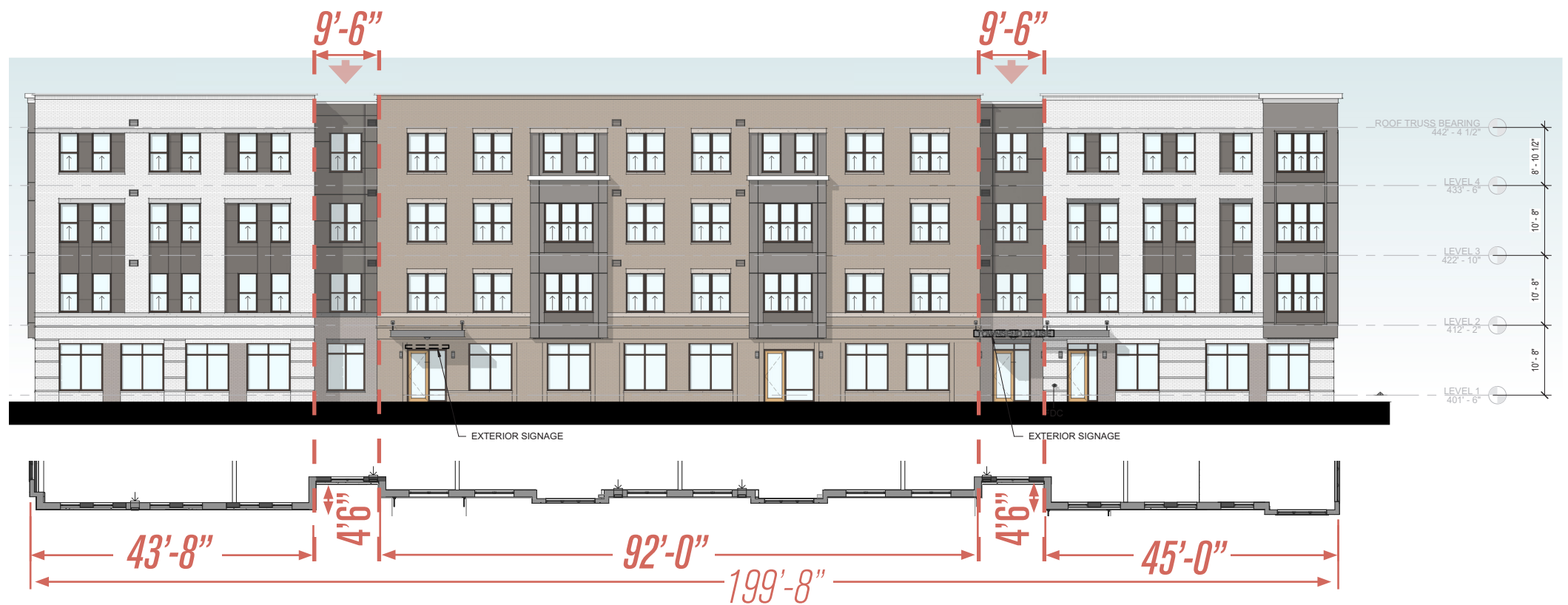
ELEVATION 2 - EAST FACADE
