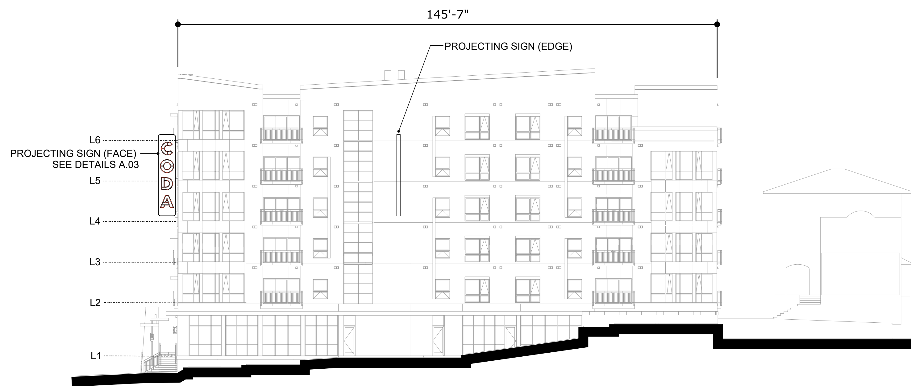
2 SOUTH ELEVATION (EAST GENESEE STREET) A.02 SCALE: 1/16" = 1' - 0"
