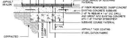
16 CITY OF SYRACUSE CONCRETE PAVEMENT - 2 POUR HEAVY DUTY NOT TO SCALE 32-313-02B
