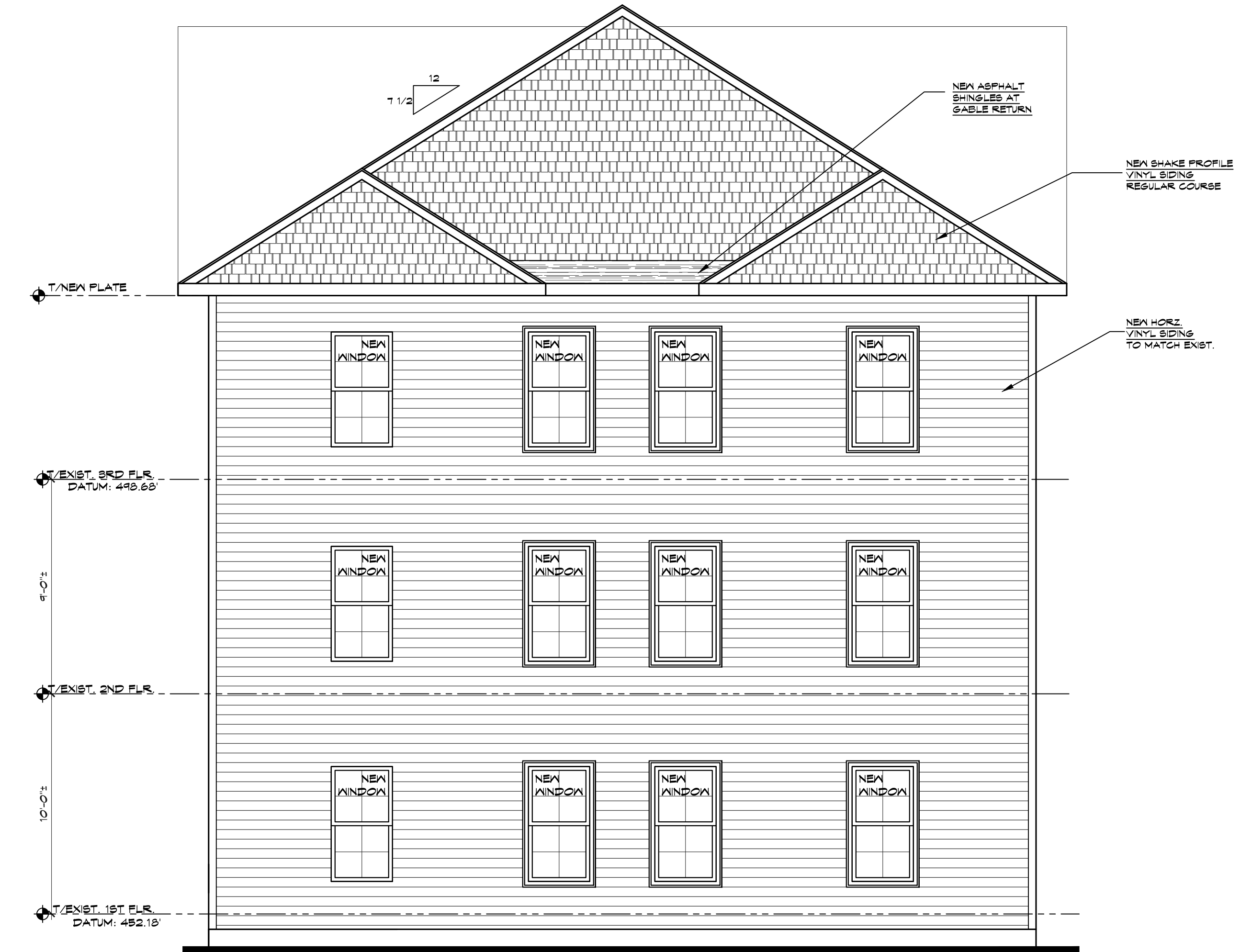
1 A-SW NEW REAR EXTERIOR ELEVATION (WEST) SCALE: 1/4" = 1'-0"
