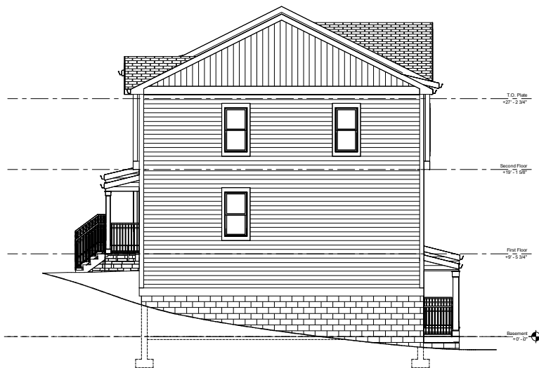
3 Duplex Side Elevation 1 1/8" = 1'-0"
