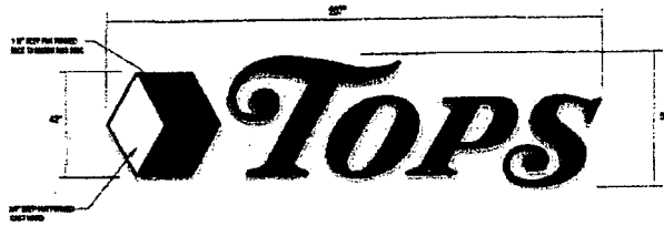
1 TOPS-54CL CHANNEL LETTER LAYOUT 77.82 SQ. FT. SCALE: 3/8" = 1'-0"
