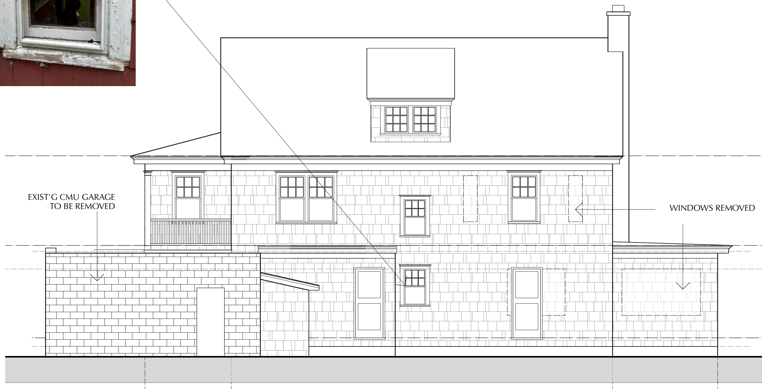
EXISTING EAST ELEVATION
