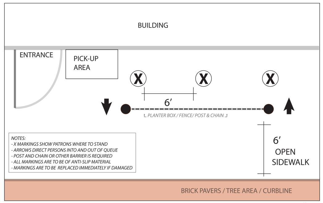
NOT TO SCALE CONCEPTUAL DRAWING ONLY SITE CONDITIONS AND LAYOUT MAY VARY MARK CORNERS OF QUEUING AREA WITH GAFFER TAPE ON SIDEWALK TO DELINEATE BOUNDARY.
