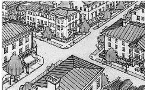
T5 areas have more mixed uses, taller buildings (3 to 6 stories), and buildings pulled closer to the street.
